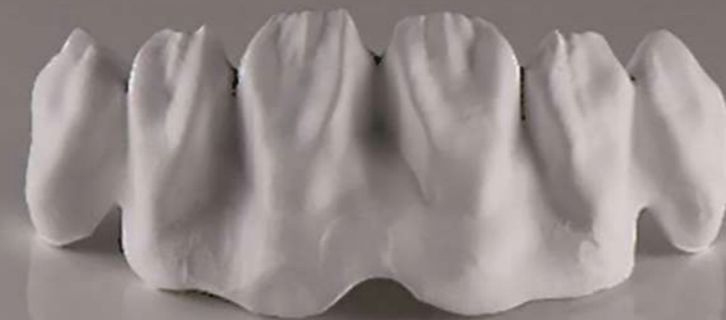
Figure 1 KATANA™ Zirconia HTML Plus (A2 shade) structure immediately after milling.
