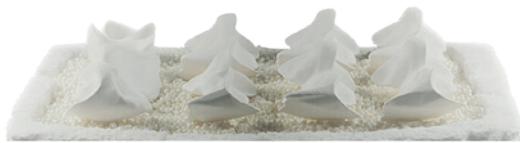
Alumina sintering beads may be the cause of white spots on a restoration surface if not replaced on a regular basis.
