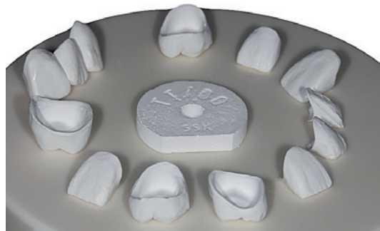
TempTAB on a sintering tray with restorations ready for sintering.
