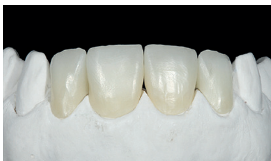
Effect of temperature differences during sintering on restorations made of "KATANA™ Zirconia" UTML: The restorations were sintered at the same nominal temperatures in three different furnaces!
