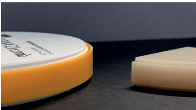
KATANA™ Multilayer HTML before (left) and after sintering.
