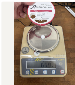
KATANA YML — 6.58 g. The milled sphere, weighed.
