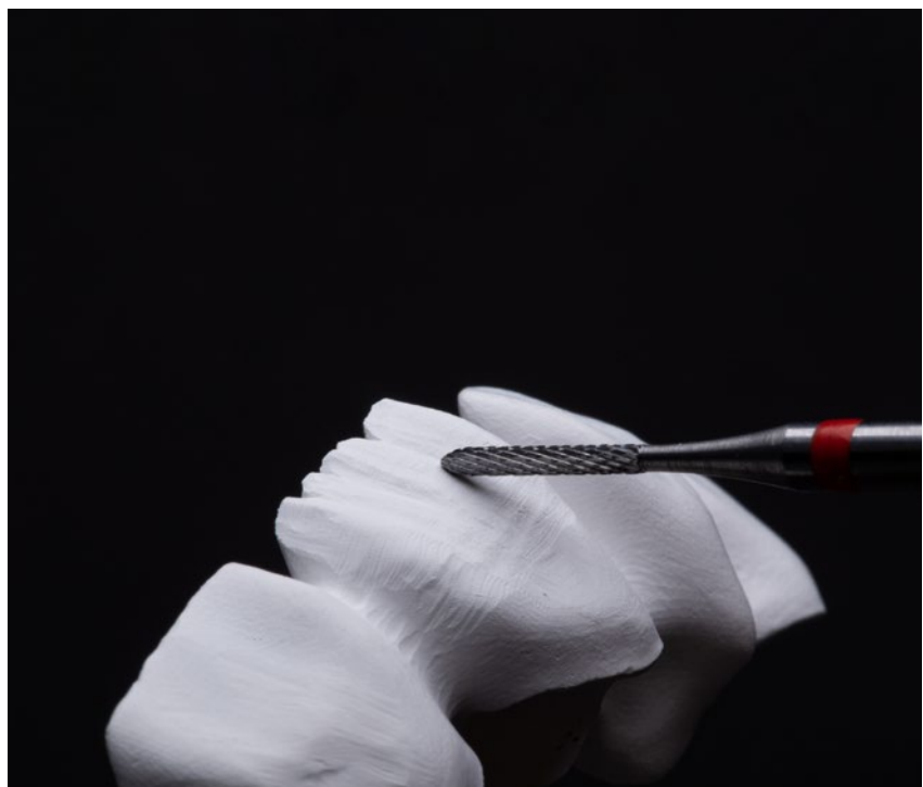
FIG. 06 Vestibular and incisal reduction and surface texturing on the pre-sintered restorations made of KATANA™ Zirconia.
