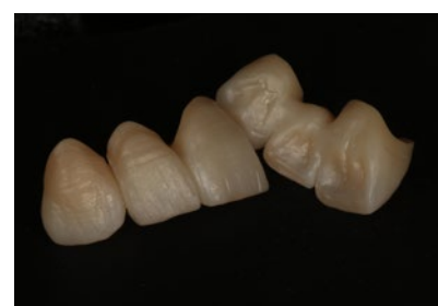
FIG. 10 Appearance of the restorations immediately after sintering.
