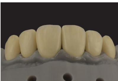
FIG. 15 Monolithic zirconia restorations on the resin model after the 7-hour final sintering.
