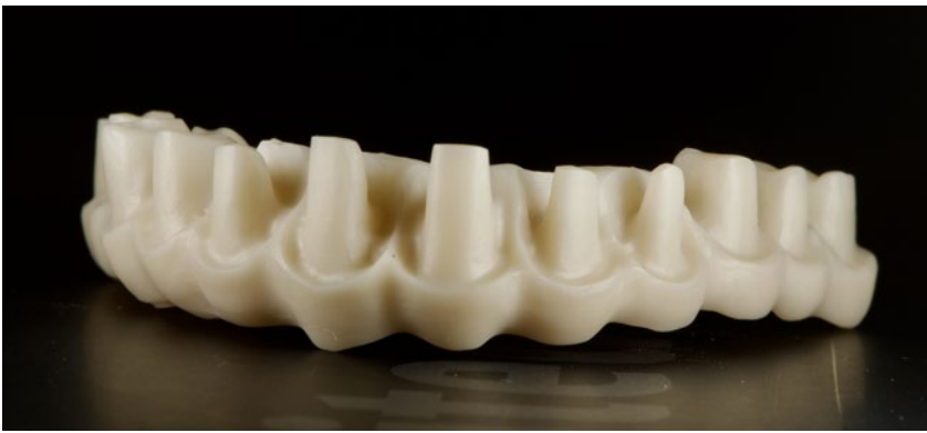
FIG. 01 Sintered bar milled from KATANA™ Zirconia HTML Plus..
