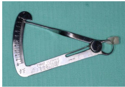
FIG. 6B Interproximal thickness: 0.5 mm
