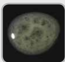
iBond™ Self Etch - phase separation Inhomogenous bond reducing bonding performance
