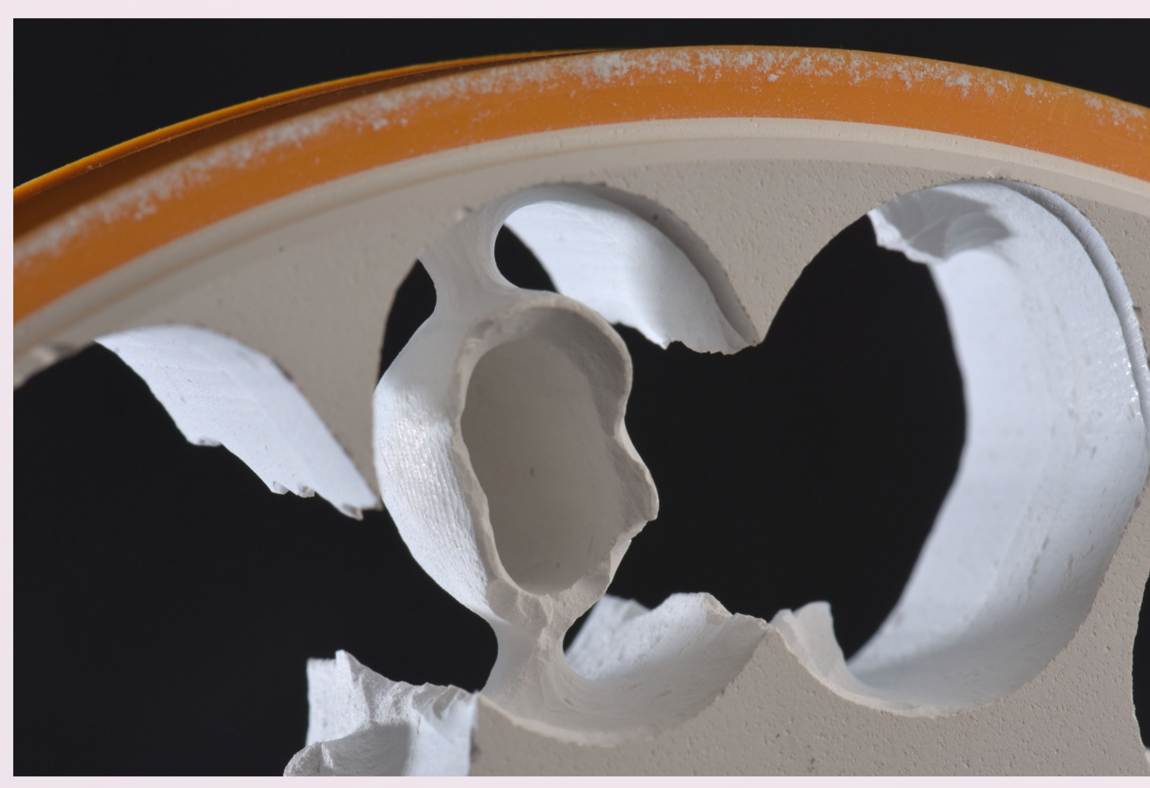
Damaged restoration on removal from the milling machine.
