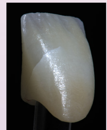
Anterior crown with a micro-cutback and a crack that might have been induced during milling.
