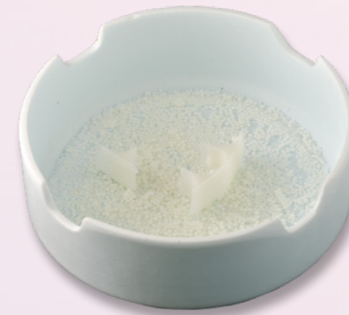
Residual pieces of non-shaded high-translucency zirconia placed in a sintering tray on sintering beads for furnace decontamination.
