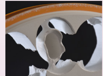
Damaged restoration on removal from the milling machine.
