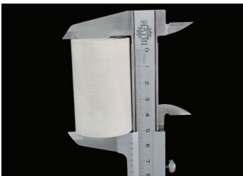
Carefully level the ring so that the top and bottom are perpendicular to the sides of the ring.
