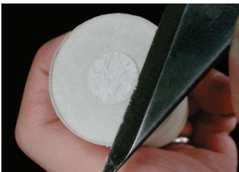
Remove the button of investment created by leveling cap
