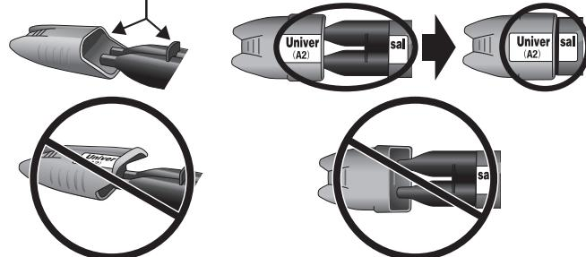
If the direction of the replaced cap is incorrect, Paste A might come into contact with Paste B at the tip of the syringe. When the heterogeneous pastes contact each other, the contacted portion of the pastes will cure.
