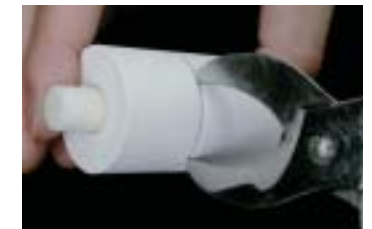
Final removal with a plaster nipper
