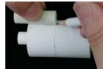
Marking the top position of the plunger
